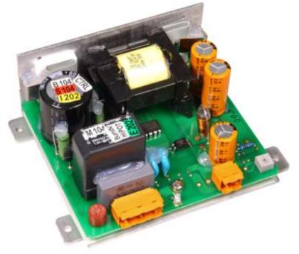
Single-Output: 24V, 36V, 48V, 60V, 72V, 140V
