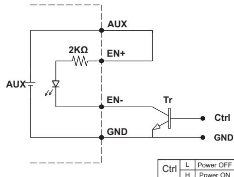
(B) ON / OFF Control by NPN transistor
