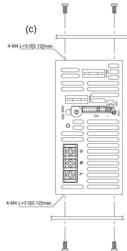
Recommended screw length is measured from the power supply surface
