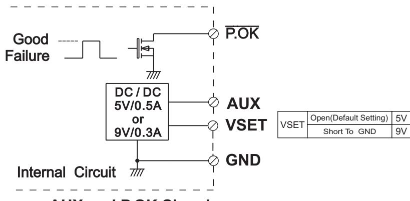
\*Place an additional capacitor to have a better performance of auxiliary power operation.
