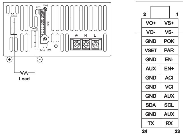
VS-, VS+ Compensation Voltage < 0.5V
