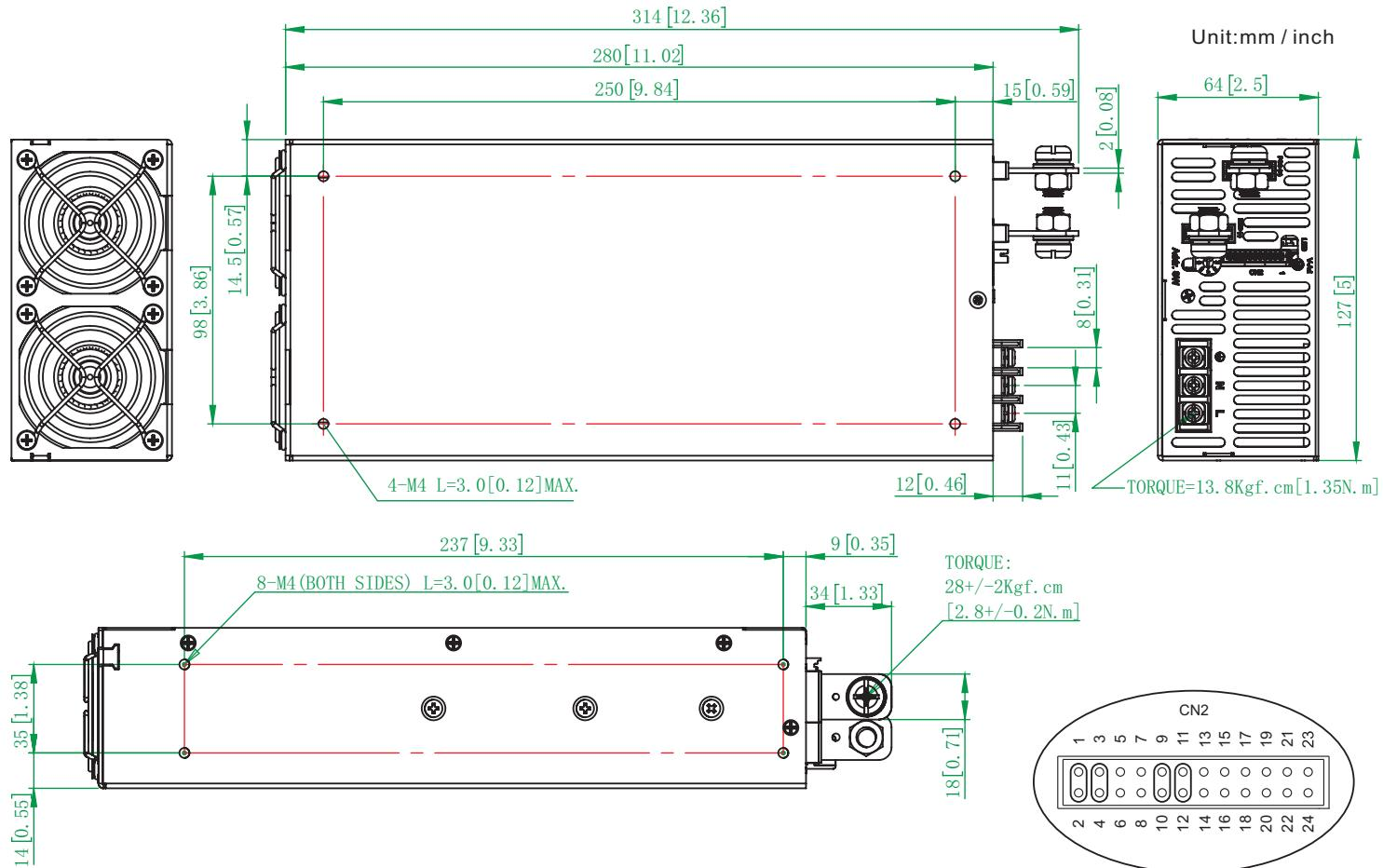
Recommended screw length is measured from the power supply surface
