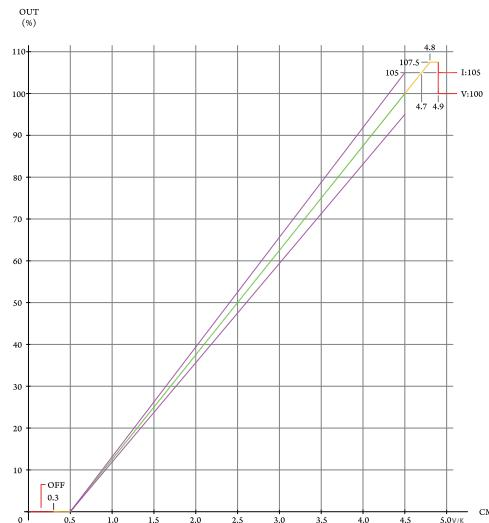
To ensure the power supply output voltage and current could be accurately adjusted, please make sure to adjust the output voltage and current > 10% vs. the rated voltage and current. (e.g. for a 24V unit, please adjust the DC output voltage above 2.4V to ensure accuracy; same applies to the output current)
