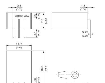
Dimensions in mm (inch) Tolerances:  $x.x \pm 0.5 (\pm 0.02)$
