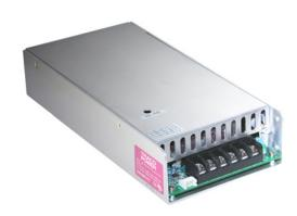
The TXH 600 series models are very compact 600 Watt universal power supplies. Rear side IEC-C13 line socket including mains switch and fuse and the output screw terminal make the connection of these power supplies very easy. Sense line, auxiliary output, remote control, adjustable output voltage, and current share line for up to 3 units in parallel make the units all-purpose applicable.
