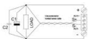
**Remote Sensing (2V per lead load, fig6)**
