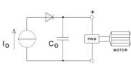
Conventional power supply: braking power charges output capacitor C<sub>o</sub>
