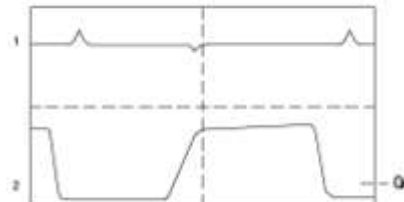
Dynamic reaction of power sink equipped power supply: load current switches between positive and negative
