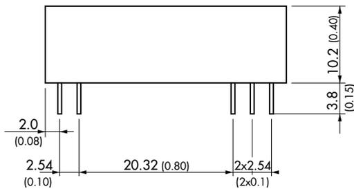
Optional pinning with options: suffix **-B1** (alternative pinning); **-B2** (with Trim); **-B3** (with Remote); **-B4** (with Trim and Remote)
