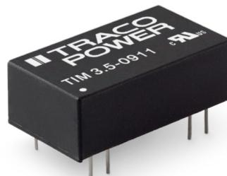
The TIM 3.5 series is a range of 3.5 Watt DC/DC converters in compact DIP-16 package and with reinforced isolation of 5000 VACrms for medical applications. With a low leakage current of less than 2 µA the converters are predestined to insulate electrical equipment from the applied parts to patient (BF classification). The models are approved to IEC/EN/ES 60601-1 3rd edition for 2×MOPP up to an altitude of 5000m and come along with an ISO 14971 risk management file.
