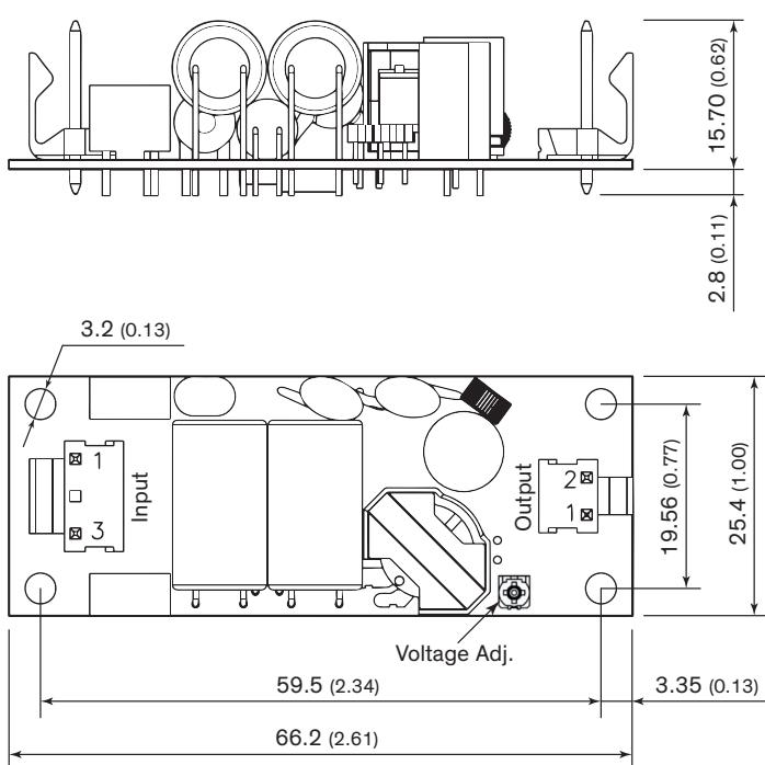
Each one of the 4 screw holes can be used as a PE connection for class I applications
