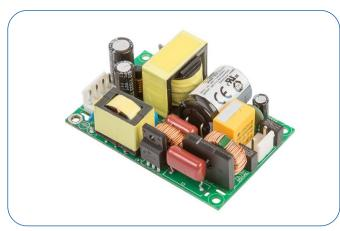
The ECP130 series is designed to minimize the no load power consumption and maximize efficiency to facilitate equipment design to meet the latest environmental legislation. Approved for medical and ITE applications, this range of single output AC-DC power supplies are packaged in a low profile 1.1" height with a foot print of just 2" by 3". The ECP130 provides up to 130 W force-cooled or | 100 W convection-cooled leading to very high power densities of 19.7 W/in³ or 15.1 W/in³ respectively.
