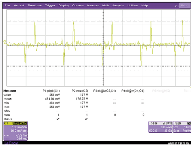
5 V/40 A Module, 50 to 100% load Change
