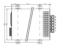
Max. terminal screw locked torque: 0.7 Nm Max. mounting screw locked torque M3: 0.8 Nm Max. mounting screw locked torque M4: 1.6 Nm
