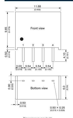
Dimensions in mm (inch) Tolerances:  $x.x \pm 0.5 (x.xx \pm 0.02)$  $x.xx \pm 0.25 (x.xxx \pm 0.01)$ Pin dimension tolerance: ±0.1 (±0.004)
