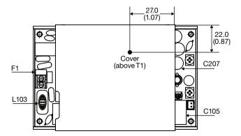
In order to ensure safe operation of the PSU in the end-use equipment, the temperature of the components listed in the table must not be exceeded. Temperature should be monitored using K type thermocouples placed on the hottest part of the component (out of direct air flow).
