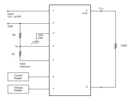
Operate with 5VDC Reference Voltage Variable output
