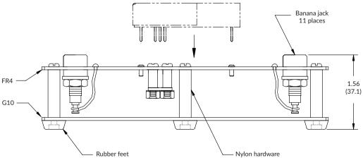
This FS-EB evaluation board provides a convenient package to use any FS Series high voltage power supply without having to it onto a PC board. The board provides for easy prototyping and evaluation. Please note when ordering, the FS Series unit is not included and must be ordered separately.
